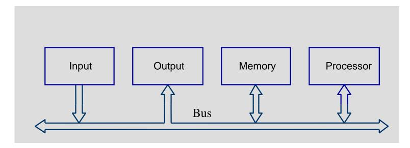
•Functional units may be connected by a group of parallel wires.
