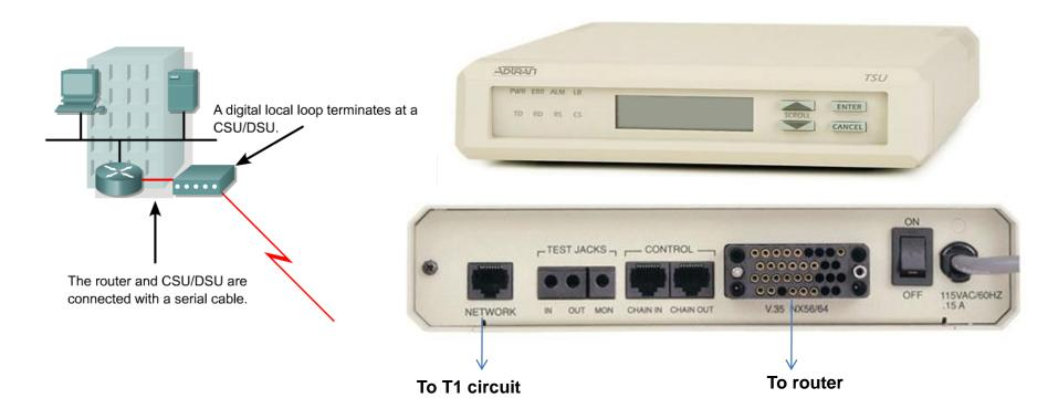
For digital lines, a **channel service unit (CSU)** and a **data service unit (DSU)** are required. We won't go into the differences here. The two are often combined into a single piece of equipment, called the **CSU/DSU**.
