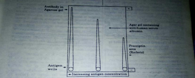
Fig. 7: Rocket electrophoresis. Antigen, in this case human serum albumin, is electrophoresed into gel containing antibody. The distance from the starting well to the front of the rocket-shaped arc is related to antigen concentration. In the example shown, human serum albumin is present at relative concentrations from left to right: 3:2:1.
