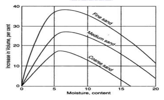
A fully saturated fine aggregate does not show any bulking. The rate of bulking is inversely proportional to the size of the aggregates. Hence, fine aggregates bulk more compared to coarse aggregates.
