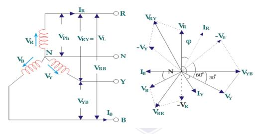
Suppose due to load impedance the current lags the applied voltage in each phase of the system by an angle  $\phi$ . As we have considered that the system is perfectly balanced, the magnitude of current and voltage of each phase is the same. Let us say, the magnitude of the voltage across the red phase i.e. magnitude of the voltage between neutral point (N) and red phase terminal (R) is  $V_R$ .
