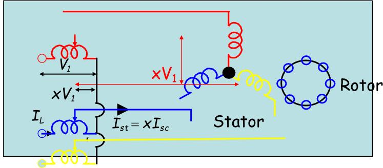
Line current at input due to auto-transformer starting <sub>=X</sub> Line current at input due to stator reactor starting <u>Starting torque with auto transformer starting</u><sub>=1</sub> Starting torque with stator reactor starting
