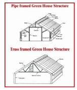
iron is welded together to form a truss encompassing rafters, chords and struts (Fig. 4). Struts are support members under compression and chords are support members under tension. Angle iron purlins running throughout the length of greenhouse are bolted to each truss. Columns are used only in very wide truss frame houses of 21.3 m or more. Most of the glass houses are of truss frame type, as these frames are best suited for prefabrication.
