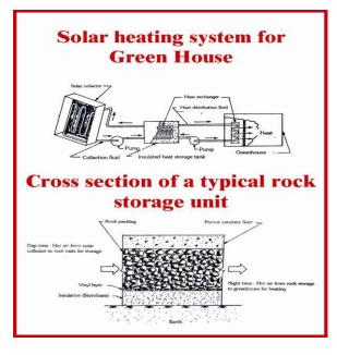
temperature rise of 17°C above the ambient condition is expected during the daytime in solar storage units. Each kilogram of water can supply 71.1 kJ of heat, and each kilogram of rock cansupply14.2 kJ of heat, as it cools by 17°C.
