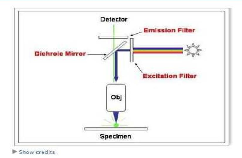
•The refinement of epi-fluorescent microscopes and advent of more powerful focused light sources, such as lasers, has led to more technically advanced scopes such as the confocal laser scanning microscopes (CLSM) and total internal reflection fluorescence microscopes (TIRF).
