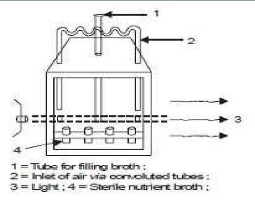
Figure 4: Dust free chamber designed by John Tyndall
