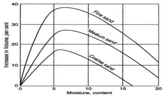
A fully saturated fine aggregate does not show any bulking. The rate of bulking is inversely proportional to the size of the aggregates. Hence, fine aggregates bulk more compared to coarse aggregates.
