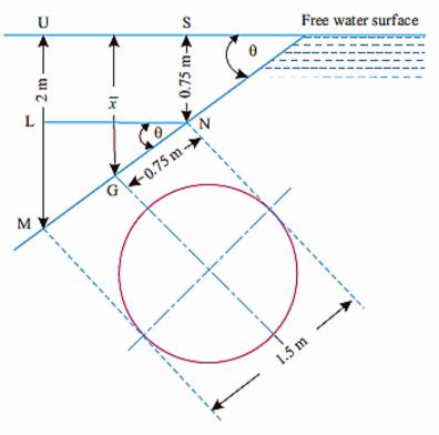
A triangular plate of 1 metre base and 1.5 metre altitude is immersed in water. The plane of the plate is inclined at 30° with free water surface and the base is parallel to and at a depth of 2 metres from water surface. Find the total pressure on the plate and the position of centre of pressure.
