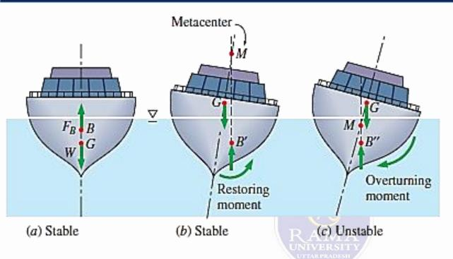
A floating body is *stable* if the body is (a) bottomheavy and thus the center of gravity G is below the centroid B of the body, or (b) if the metacenter M is above point G. However, the body is (c) *unstable* if point M is below point G.
