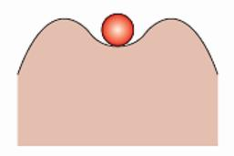
A ball in a trough between two hills is stable for small disturbances, but unstable for large disturbances
