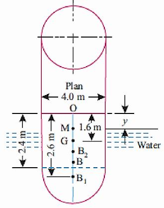
Distance of the centre of buoyancy of the cylindrical portion from the top of the body,
