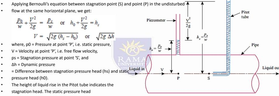
• may be measured separately with a piezometer (Fig. 6.38). Both the static pressure as well as stagnation pressure can be measured in a device known as Pitot static tube.
