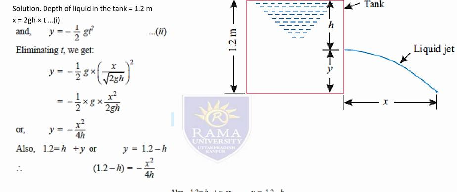
Also, 1.2=h + y or y = 1.2-h  $\therefore$   $(1.2-h) = -\frac{x^2}{4h}$ or,  $x^2 = -4h(1.2-h) = -4.8h + 4h^2$ For horizontal distance x to be maximum  $\frac{dx}{dh} = 0$  $\therefore$   $2x\frac{dx}{dh} = -4.8 + 8h = 0$  or h = 0.6 m
