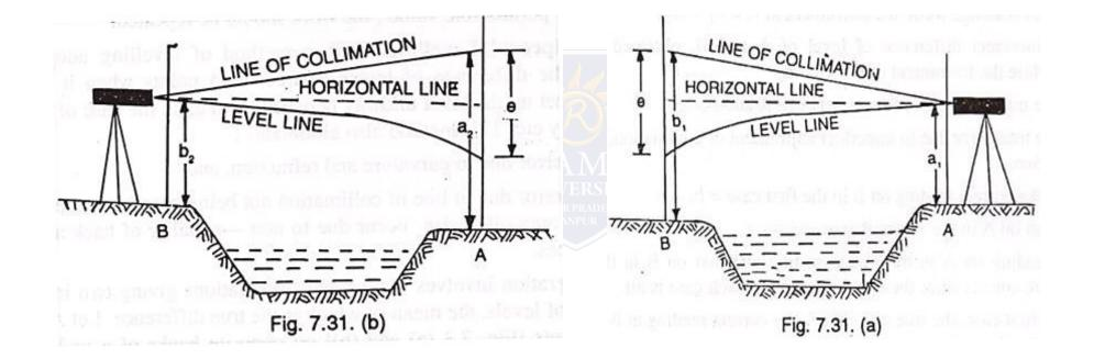
If the staff is near to the level, then the reading on it should be taken through the objectglass or the height of the centre of the eye-piece above that point should be measured directly with the staff and be considered as staff reading on that point.
