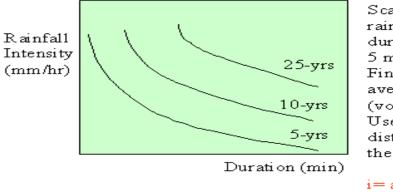
Scan the clocktime rainfall record for a duration (e.g. 5 min.); Find the maximum average intensity (volume/time); Use Extreme Type I distribution to determine the frequency
