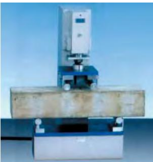
Flexural testing of concrete beam mould
