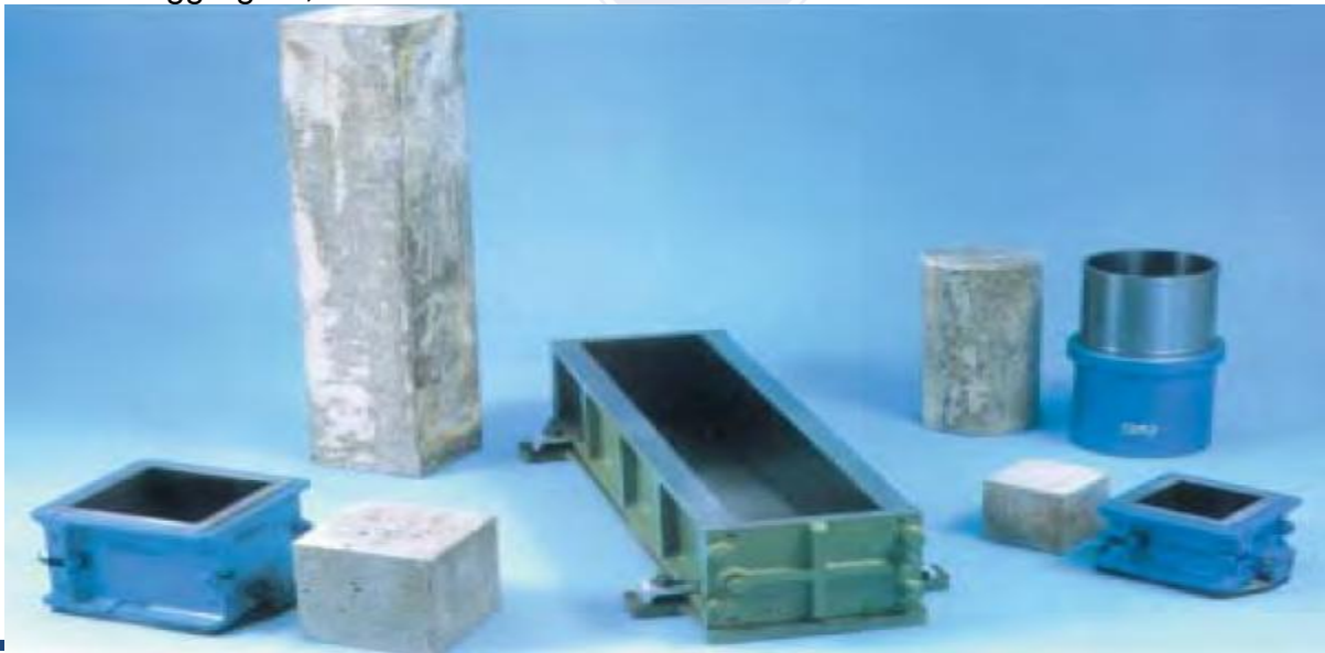
Cube beam and cylinder moulding
