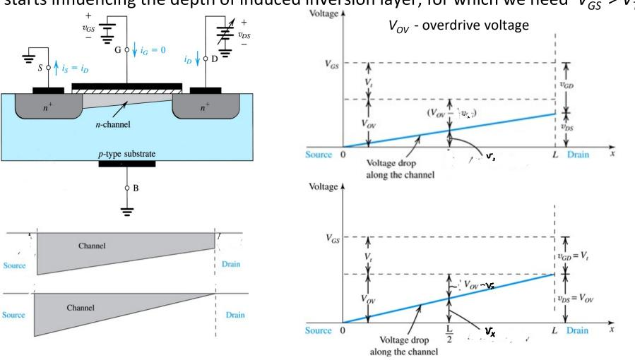
$v_{DS} = V_{OV}$  - pinch-off voltage, saturation region begins
