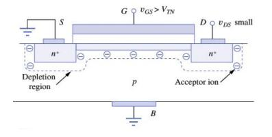
• If  $v_{DS} \lt \lt V_{GS} - V_{TN}$  MOSFET is in linear portion of the triode region
