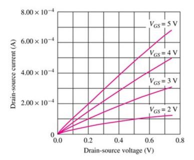
Under this condition, MOSFET behaves like a gate-source voltage-controlled resistor between source and drain,
