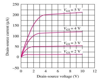
$$i_D = \frac{K'_n}{2} \frac{W}{L} \left( v_{GS} - V_{TN} \right)^2$$
