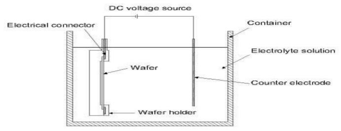
This technology is quite similar to what happens in CVD processes, however, if the substrate is an ordered semiconductor crystal (i.e. silicon, gallium arsenide), it is possible with this process to continue building on the substrate with the same crystallographic orientation with the substrate acting as a seed for the deposition. If an amorphous/polycrystalline substrate surface is used, the film will also be amorphous or polycrystalline.
