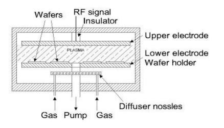
**Figure 2:** *Typical parallel-plate reactive ion etching system.*
