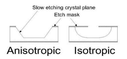
**Figure 1:** *Difference between anisotropic and isotropic wet etching*
