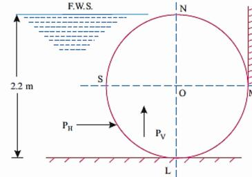
The vertical component of the resultant hydrostatic force is the weight of water supported by the curved surface LSN which represents a semicircle.  $PV = w \times volume$  of surface LSN
