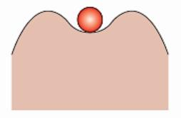
A floating body is *stable* if the body is (*a*) bottomheavy and thus the center of gravity G is below the centroid B of the body, or (*b*) if the metacenter M is above point G. However, the body is (*c*) *unstable* if point M is below point G. A ball in a trough between two hills is stable for small disturbances, but unstable for large disturbances
