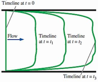
Timelines produced by a hydrogen bubble wire are used to visualize the boundary layer velocity profile shape along a flat plate. Flow is from left to right, and the hydrogen bubble wire is located to the left of the field of view. Bubbles near the wall reveal a flow instability that leads to turbulence.
