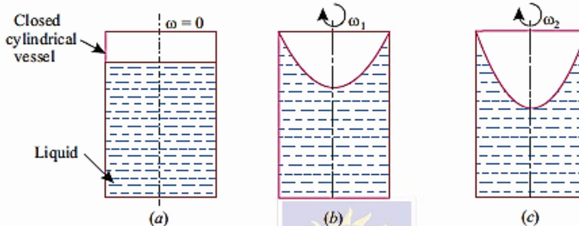
— Fig. 6.72 (a) shows the cylindrical vessel when it is stationary (i.e., it is not rotated,  $\omega = 0$ )
