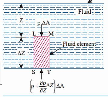
states that rate of increase of pressure in a vertical direction is equal to weight density of the fluid at that point. This is "hydrostatic law".
