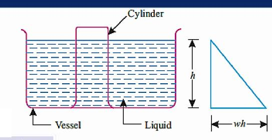
As p = wh, the intensity of pressure in a liquid due to its depth will vary directly with depth. As the pressure at any point in a liquid depends on height of the free surface above that point, it is sometimes convenient to express a liquid pressure by the height of the free surface which would cause the pressure,
