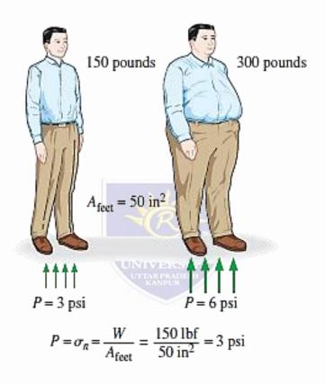
The normal stress (or "pressure") on the feet of a chubby person is much greater than on the feet of a slim person.
