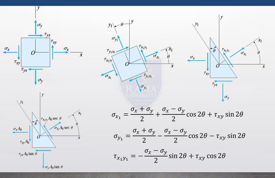
A shear stress is positive when it acts on a positive face of an element in the positive direction of an axis and it is negative when it acts on a positive face of and element in the negative direction of an axis
