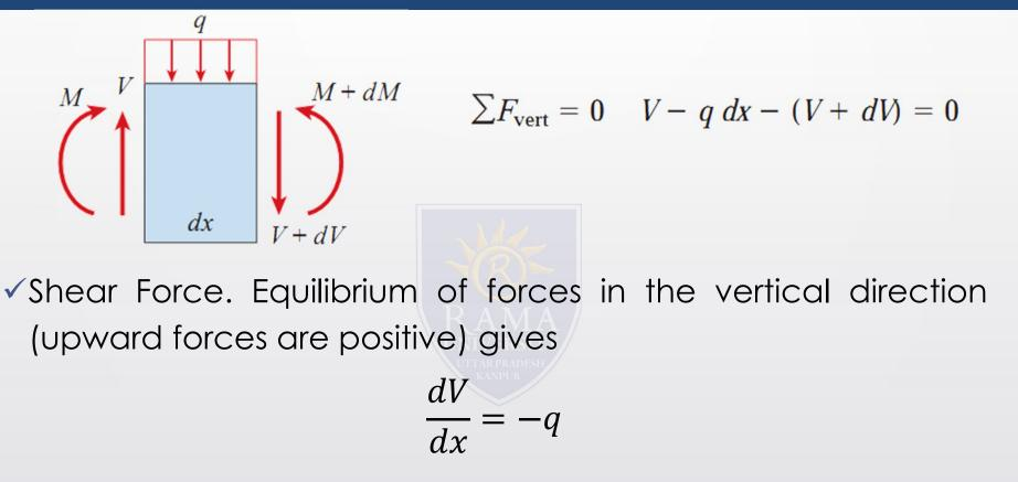
✓If the sign convention for the distributed load is reversed, so that q is positive upward instead of downward, then the minus sign is omitted in the preceding equation.
