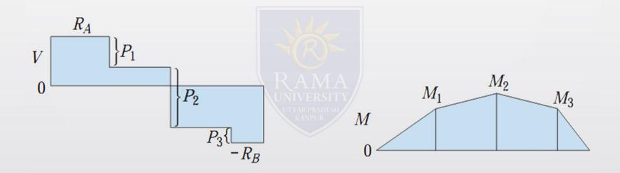
**4.5-1** Draw the shear-force and bending-moment diagrams for a simple beam AB supporting two equal concentrated loads P (see figure).
