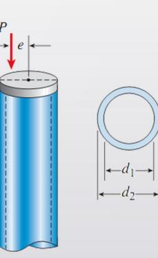
**11.5-9** The column shown in the figure is fixed at the base and free at the upper end. A compressive load P acts at the top of the column with an eccentricity e from the axis of the column.
