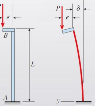
**11.6-1** A steel bar has a square cross section of width b = 50 mm (see figure). The bar has pinned supports at the ends and is 1 m long. The axial forces acting at the end of the bar have a resultant P = 80 kN located at distance e = 20 mm from the center of the cross section. Also, the modulus of elasticity of the steel is 200 GPa.
