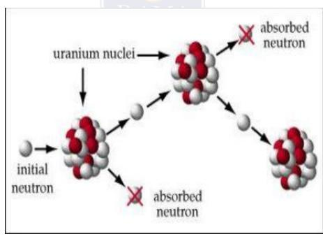
In addition to the need to capture neutrons, the neutrons often have too much kinetic energy. These fast neutrons are slowed through the use of a moderator such as heavy water and ordinary water. Some reactors use graphite as a moderator, but this design has several problems. Once the fast neutrons have been slowed, they are more likely to produce further nuclear fissions or be absorbed by the control rod.
