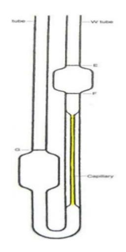
**Principle:** When a liquid flows by gravity, the time required for the liquid to pass between two marks (E and F shown in Figure) through a vertical capillary tube is determined.
