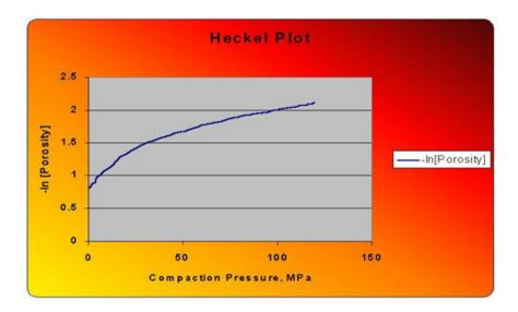
The slope of the linear regression is the Heckel constant, a material dependent parameter inversely proportional to the mean yield pressure (the minimum pressure required to cause deformation of the material undergoing compression).
